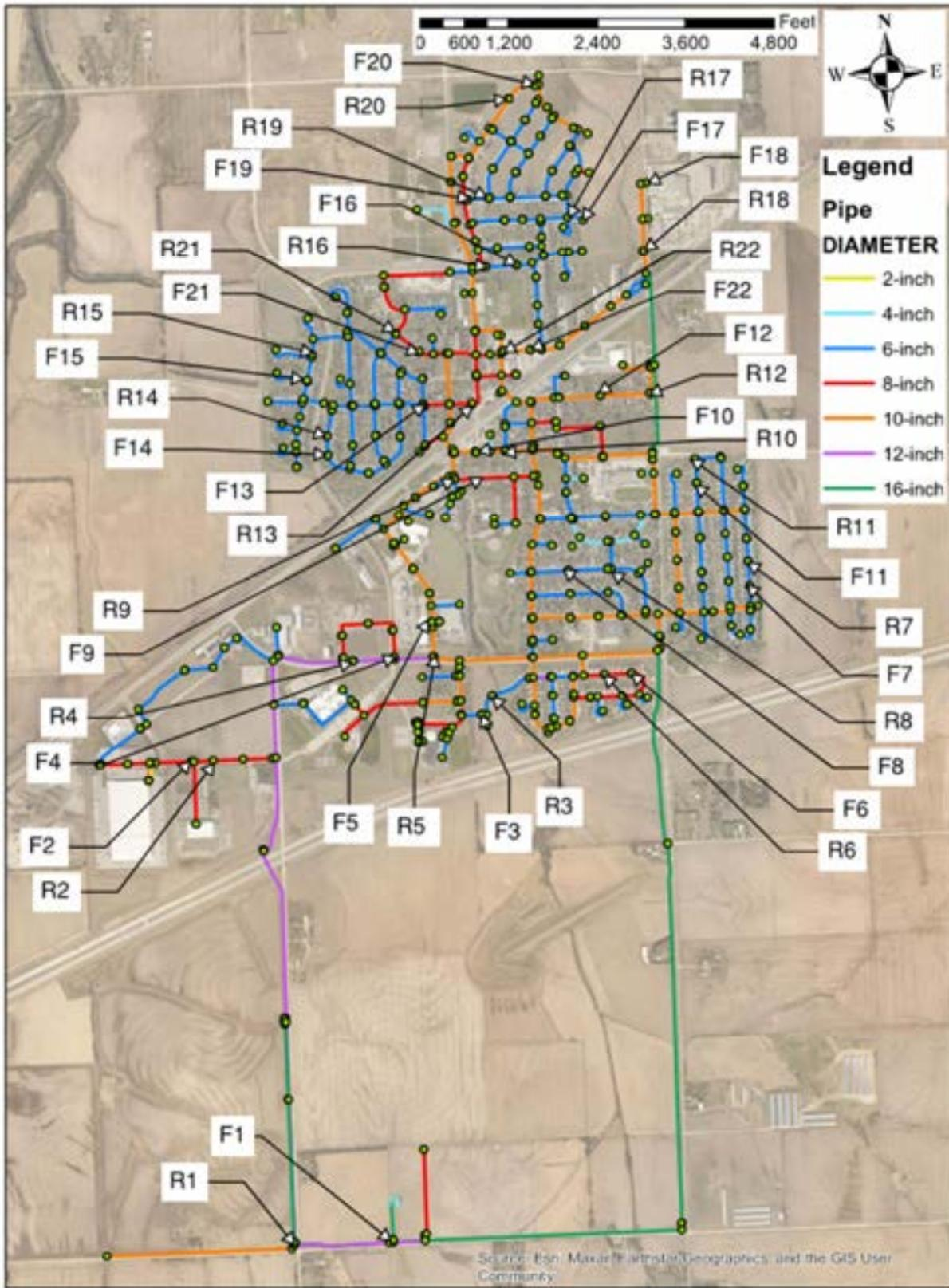
Figure 10. Flow Testing Map
