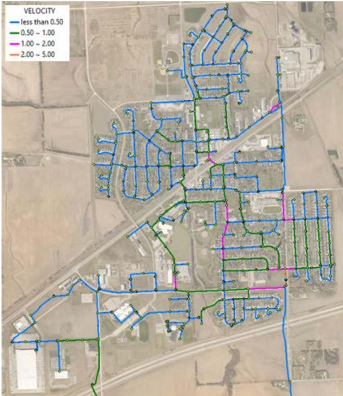
Figure 12. Pipe Velocity (in fps) at Peak Hour Demand
