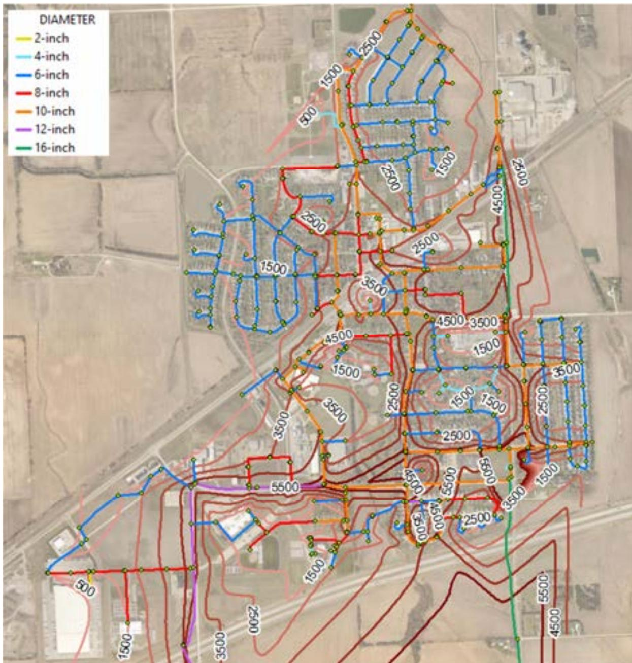
Figure 13. Fire Flow Capabilities
