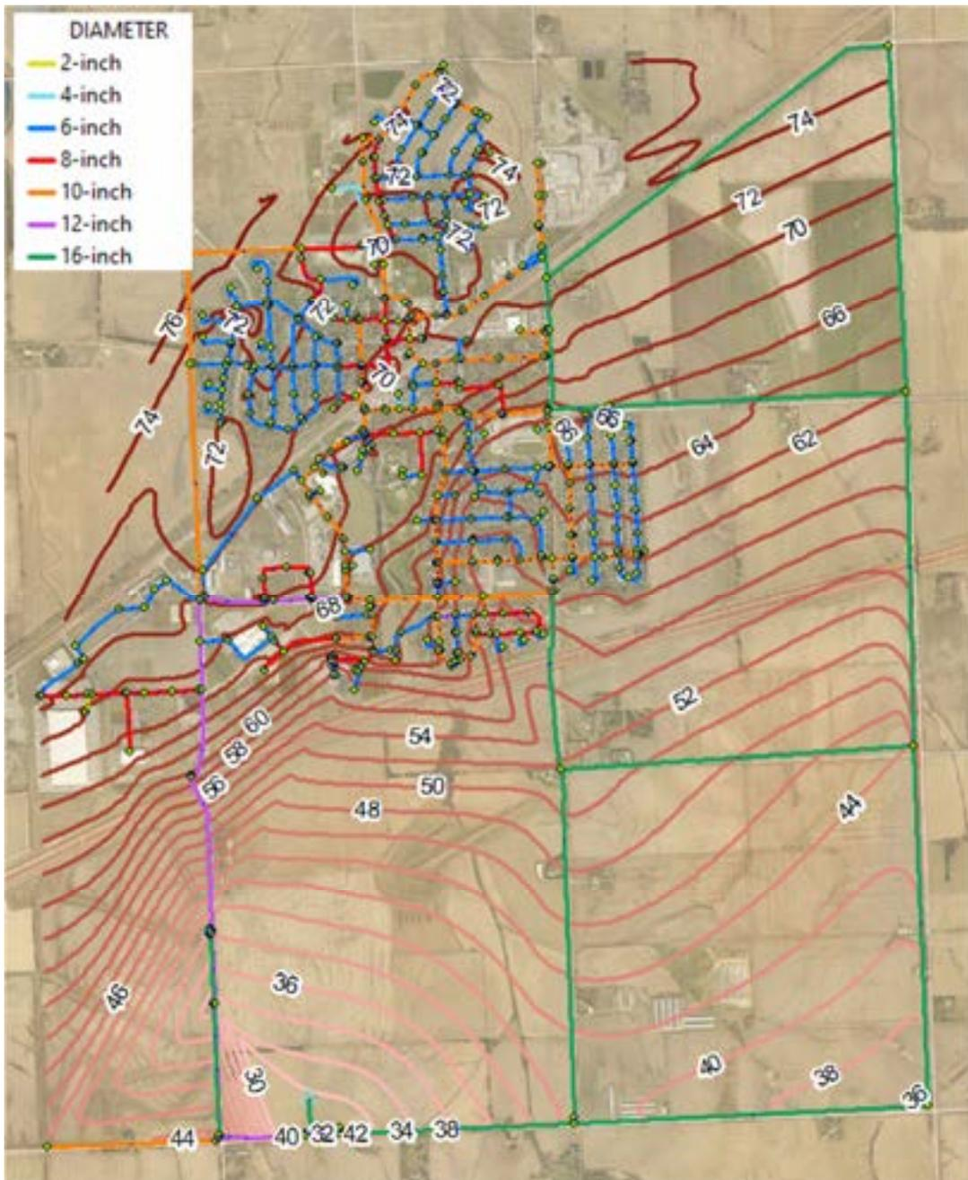
Figure 15. Pressures Around Proposed 16-inch Loop
