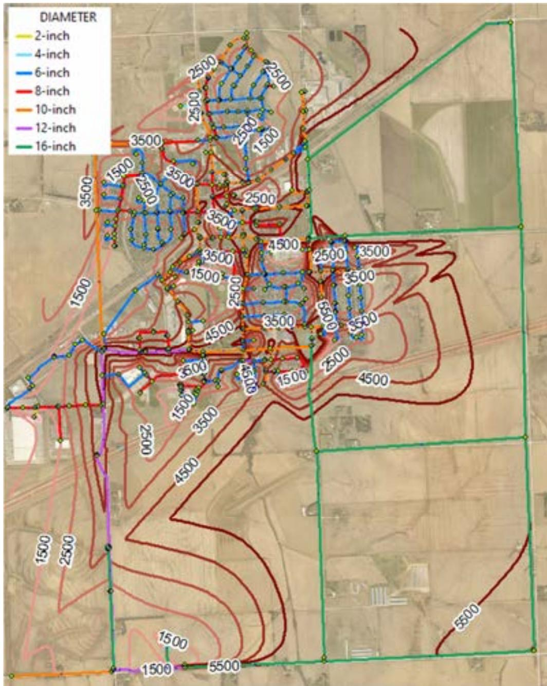
Figure 16. Available Fire Flow Around Proposed 16-inch Loop
