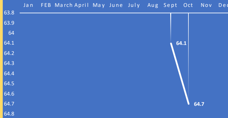
WELL #7 STATIC LEVELS 2024
