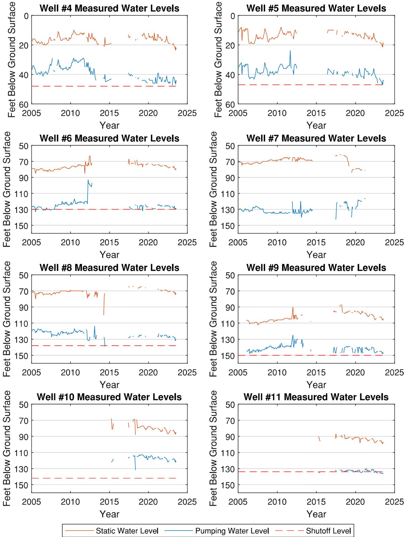
**Figure 8. Waverly municipal wells static, pumping, and shutoff water levels.**
