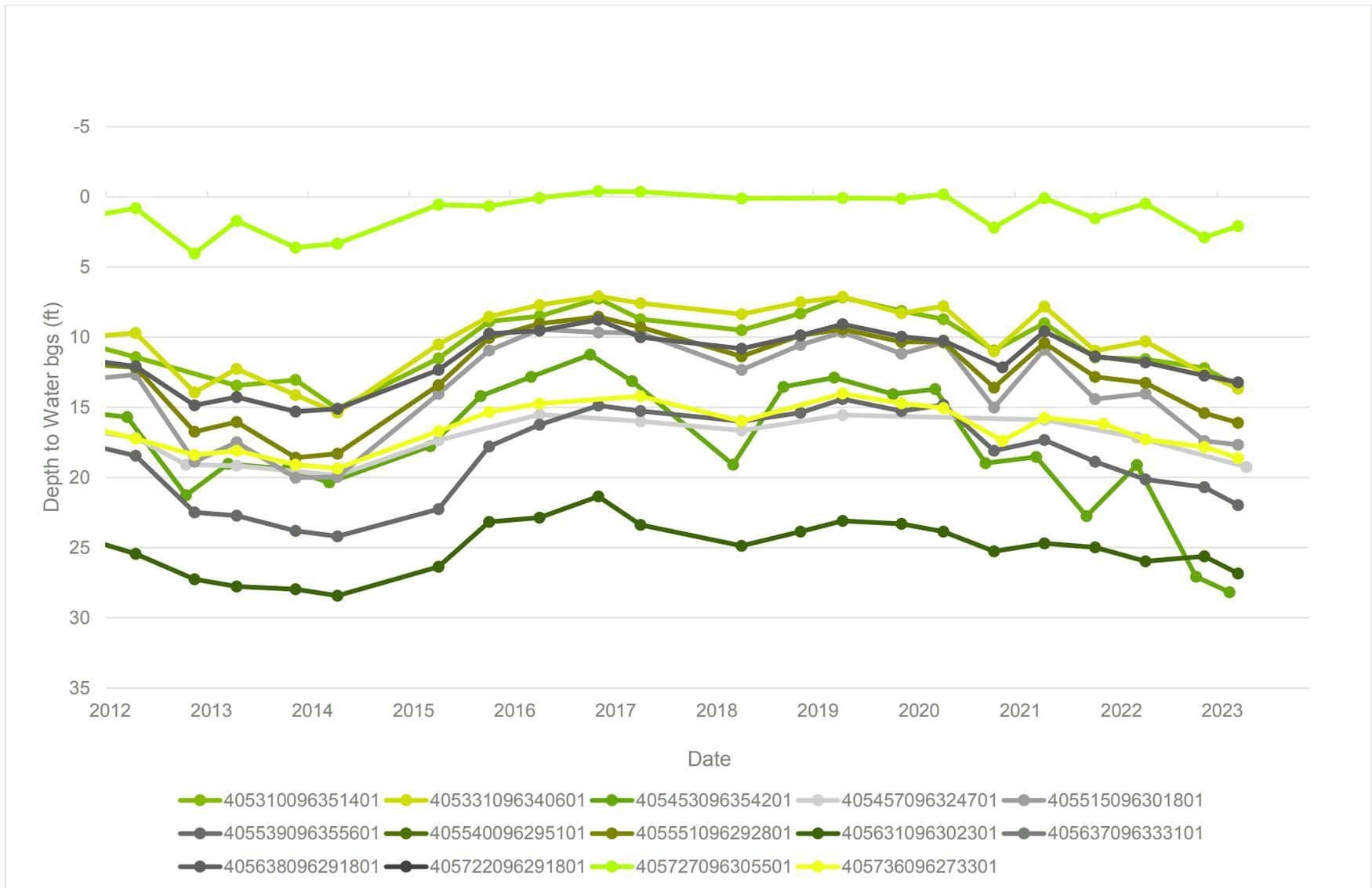
Figure 11. Depth to water below ground surface for nearby USGS monitoring wells from 2012 to 2023.
