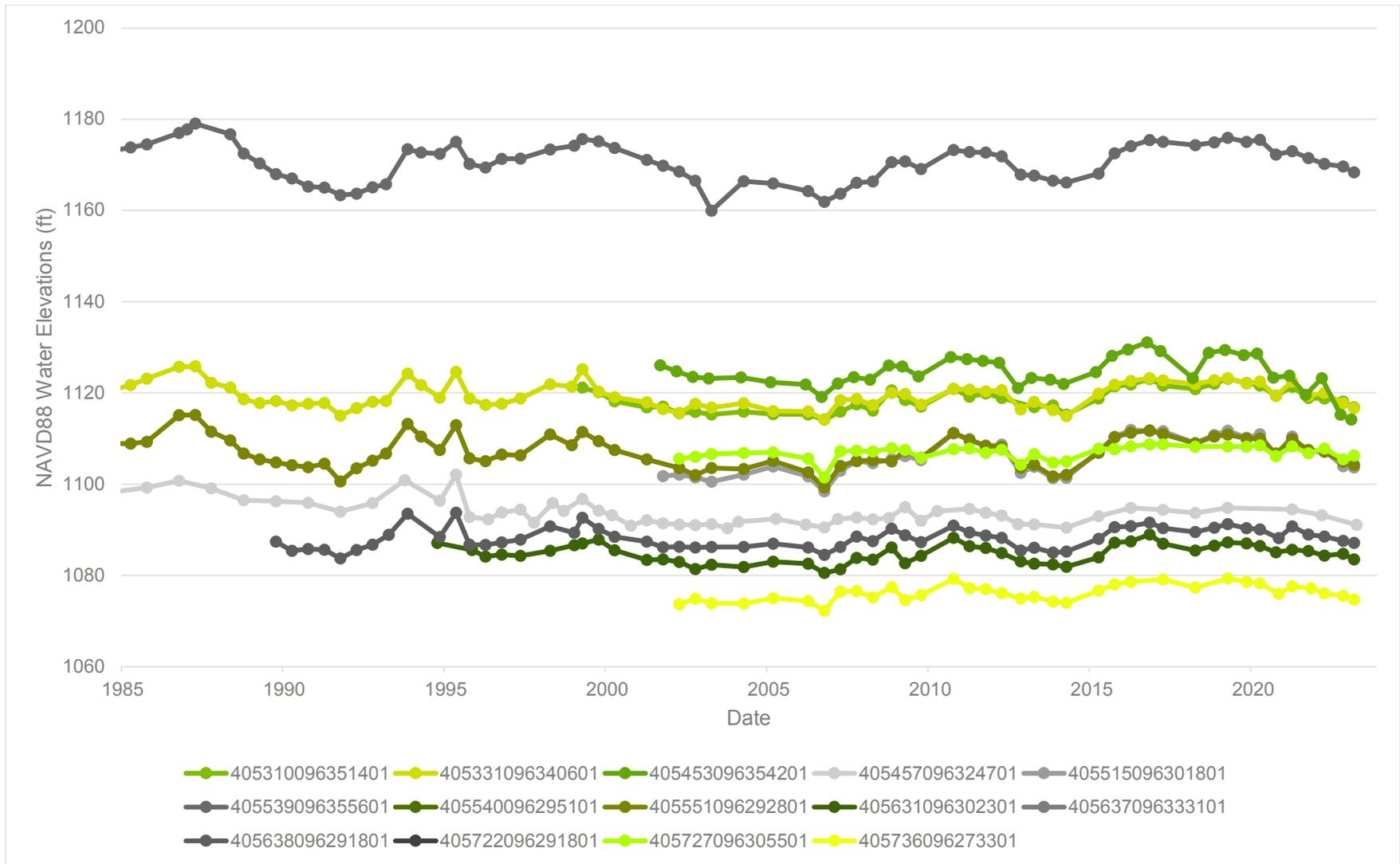
Figure 10. Water level elevations above NAVD88 for nearby USGS monitoring wells from 1985 to 2023.
